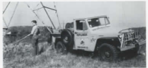
Four-wheel drive jeeps were converted for chemical brush control spraying on transmission rights-of-way.
