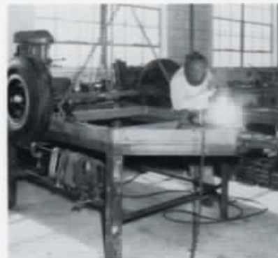
Welding chipper frame
