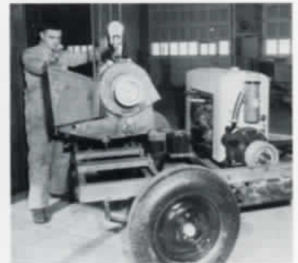
Mounting basic chipper unit and engine onto trailer frame
