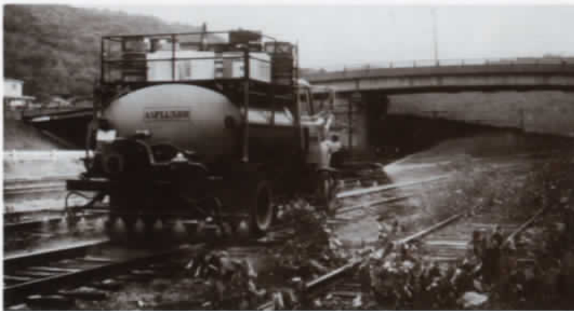
Asplundh Railroad division Hy-Rail truck quickly applies its load of herbicide, then returns to highway to reach next location.
