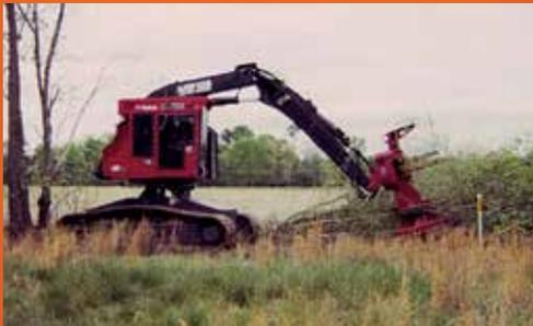
This versatile tracked feller-buncher is well suited for removing high-risk trees from the right-of-way or cutting and stacking trees during a capital clearing project.
