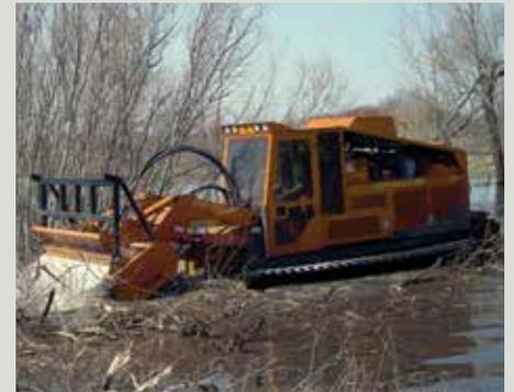
This tracked mower is ideal for cutting brush in all types of rugged or swampy terrain.
