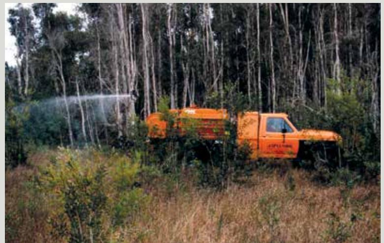
A 300-gallon truck applies a foliar herbicide using a low-drift Radiarc sprayer. Hydraulic applications include high-volume stem or foliar herbicide treatments and cut stubble applications.
