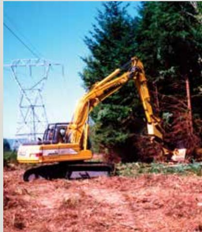
A Slashbuster unit mounted on a tracked excavator can cut and mulch whole trees or stack the trunk sections with its grapple attachment.
