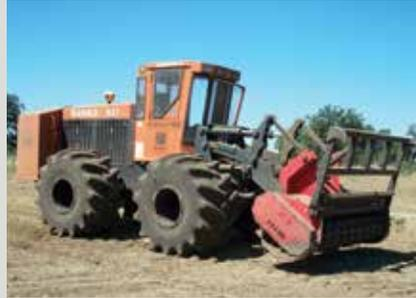
A Barko mower with a Fecon mulching head cuts and mulches brush to restore the right-of-way and prevent vegetation from interfering with conductors and towers.
