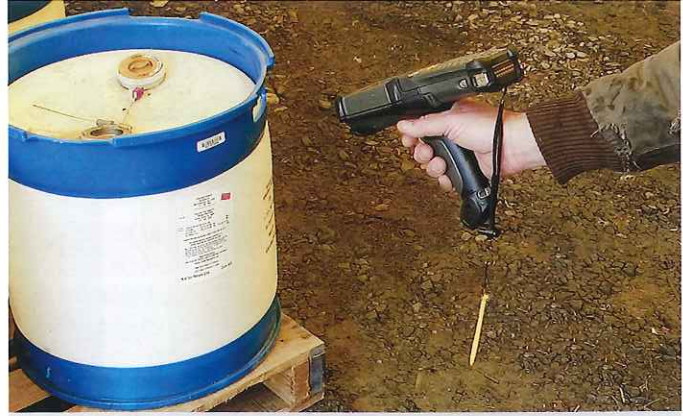
Before shipping custom-blended products to the field, a barcode scanner records identifying information on each returnable/reusable container so its movement and use can be electronically tracked. Photo by Joe Lentz
