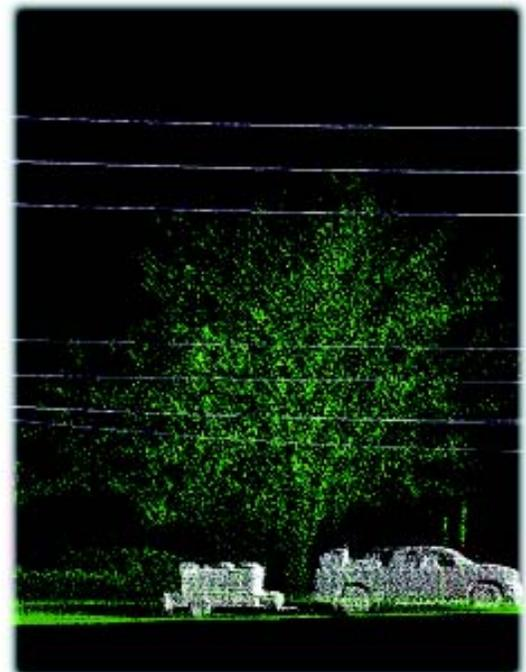
*In this URM-supplied LiDAR-generated image, the encroachment of vegetation on distribution lines can be seen.*
